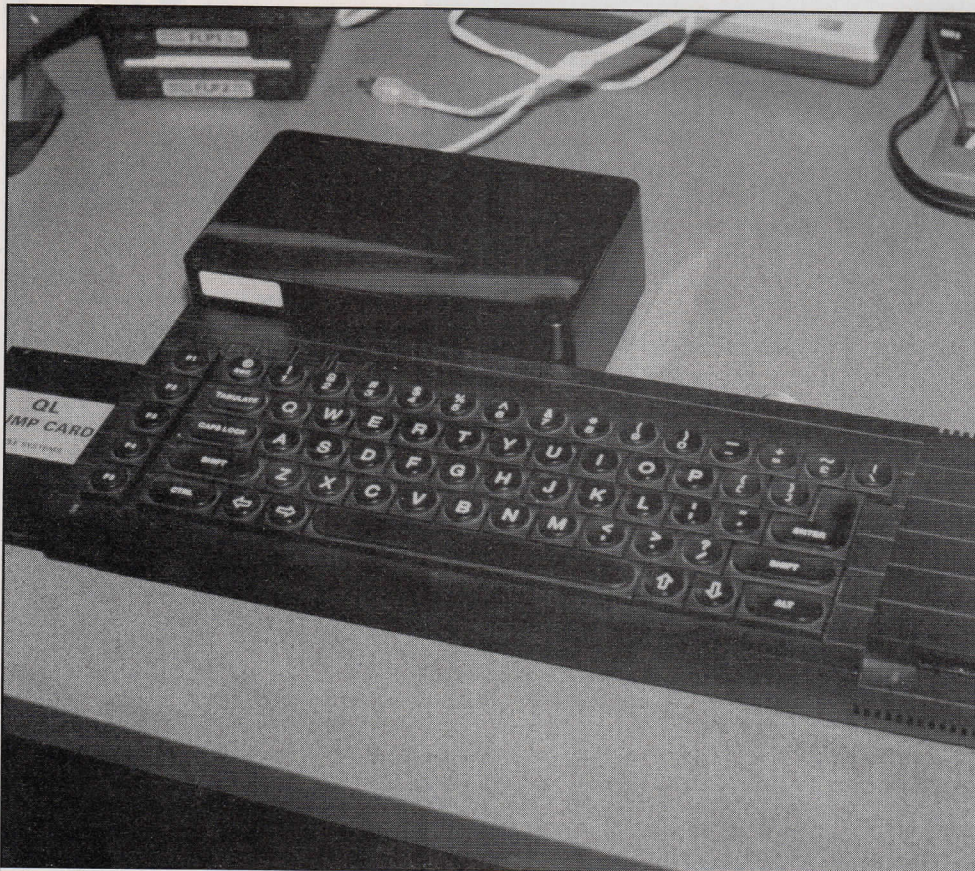
The CL digitiser connected to the QL's rom socket.
